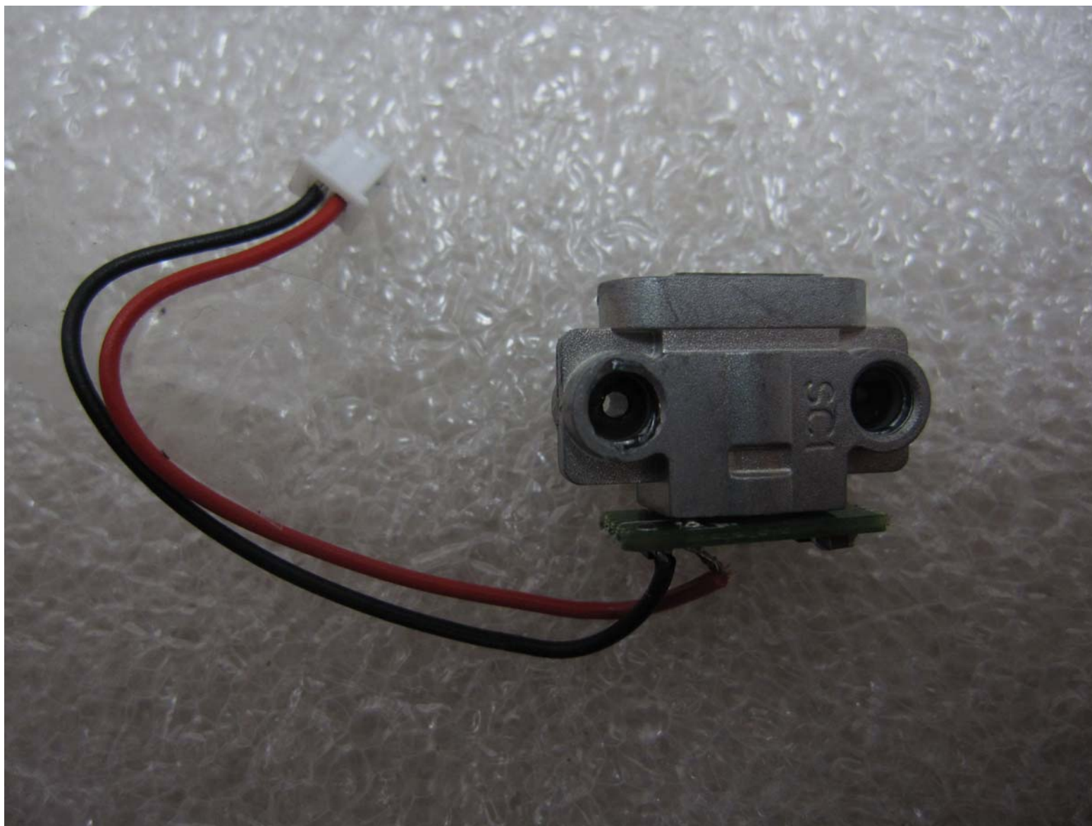
Magic Cube_Pattern Projector Module Rear
